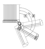
Tilting angle infinitely adjustable from 80° to 155° 1 Min. 80° 2 Max. 155° Frame hinge connector with support for keyboards
