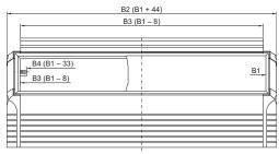
Support for keyboards SM 2383.000 for front panel width B1 = 482.6 mm
