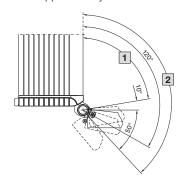
Tilting angle infinitely adjustable from 80° to 140° 1 Min. 80° 2 Max. 140°
